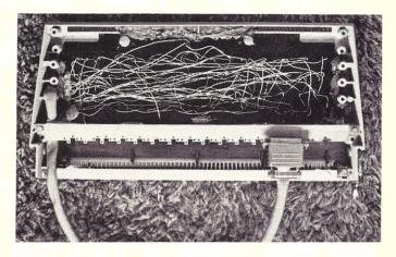
Underside of external keyboard (note silicon rubber holding the keyboard in case).
